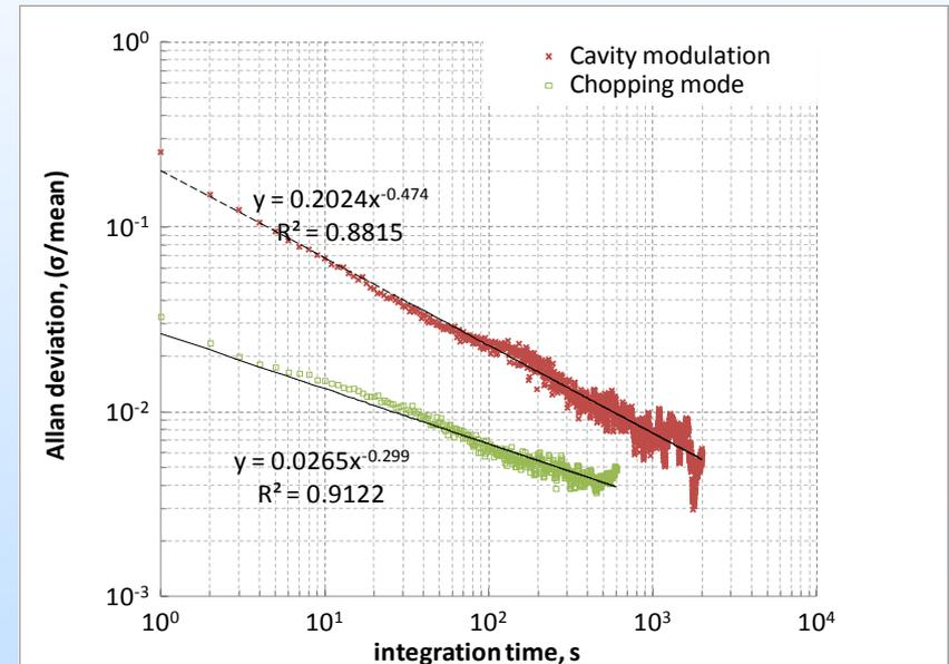
The deviation for cavity modulation (red) is shown against that of laser chopping (green) for  $^{14}\text{CO}_2$ .
