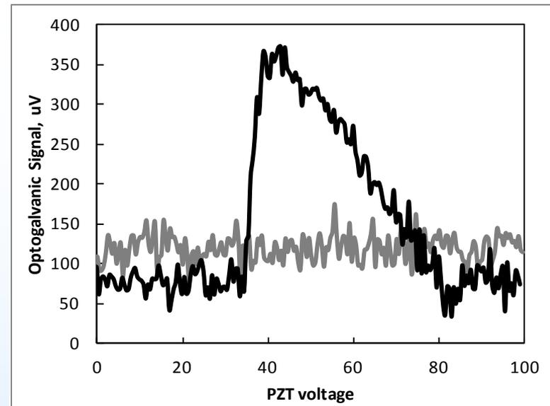
Scans do not reveal an intracavity response with cavity modulation
