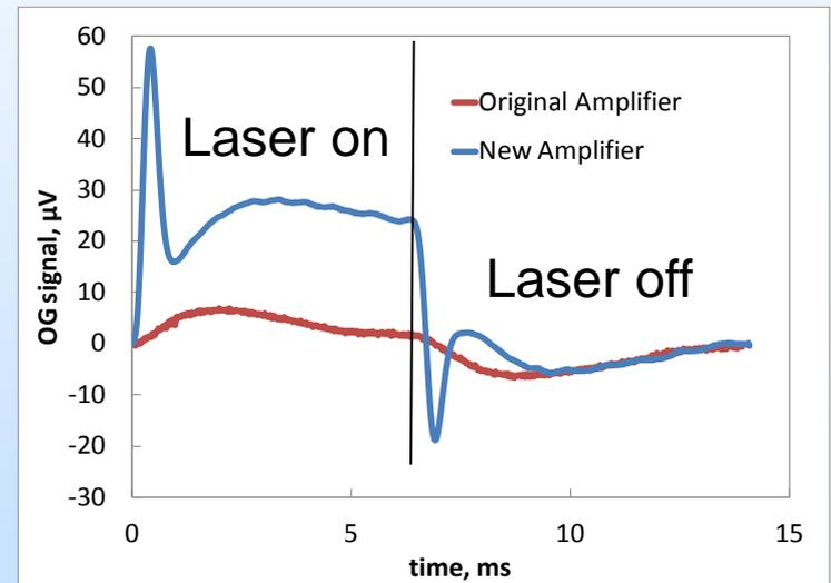
The new amplifier reveals a large transient response at short times
